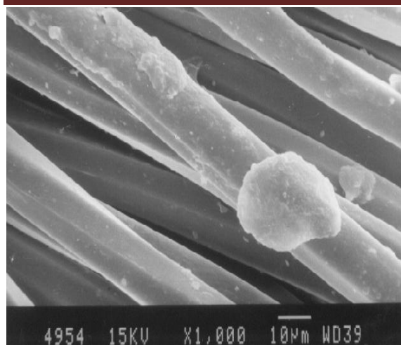
Fig.8: SEM photograph of 100% PET fabric treated with W:CTC: sBA (30 mins)
