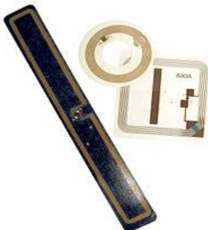
Fig. 3. Various size and shapes of RFID tags
